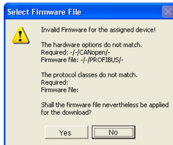
Figure 19: Request Select Firmware File - Example Invalid Firmware
